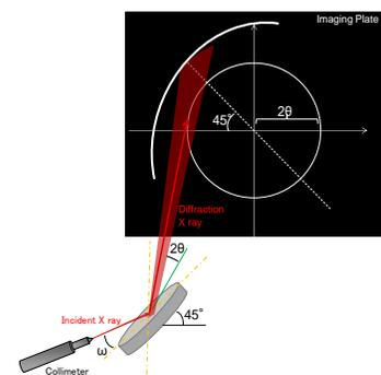
Figure 1. Geometry between incident X-ray beam angle and the sample stage in IPXRD equipment.
