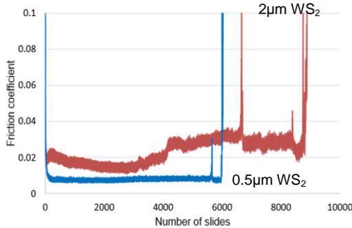
Figure 2. Friction coefficient behaviors of 0.5 $\mu\text{m}$  and 2 $\mu\text{m}$  powder  $\text{WS}_2$  in a vacuum.
