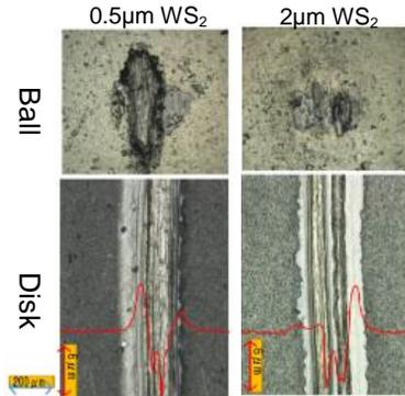
Figure 3. Microscope observation and measured surface roughness on a wear track of after friction test.
